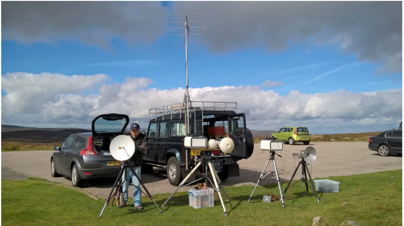
Picture shows the equipment of GW3TKH and G4HQX, from left to right, 24GHz Tvtr; together on one tripod, 76G Tvtr, 76GHz Bcn, 47GHz Tvtr; 76GHz Tvtr; 47GHz Tvtr.
