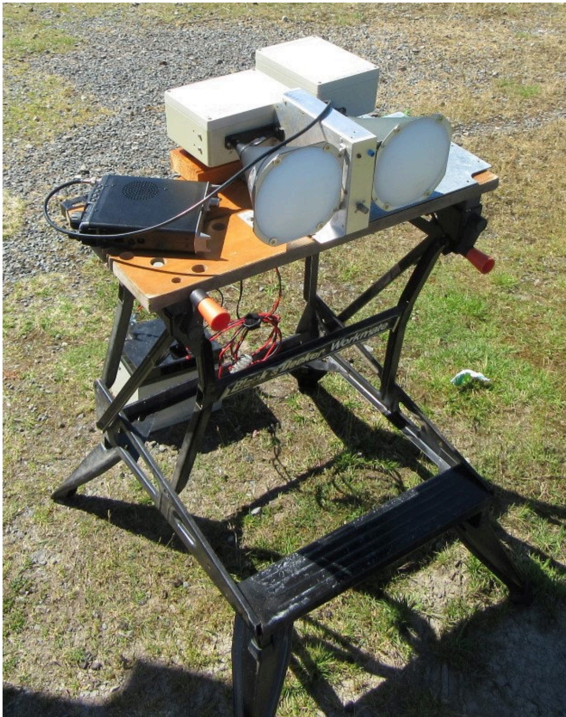
The loan 76GHz set up on a workmate, with FT817 IF.
