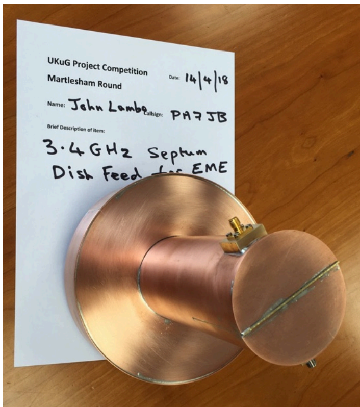
3.4GHz Septum dish feed for EME by John Lambo PA7JB
