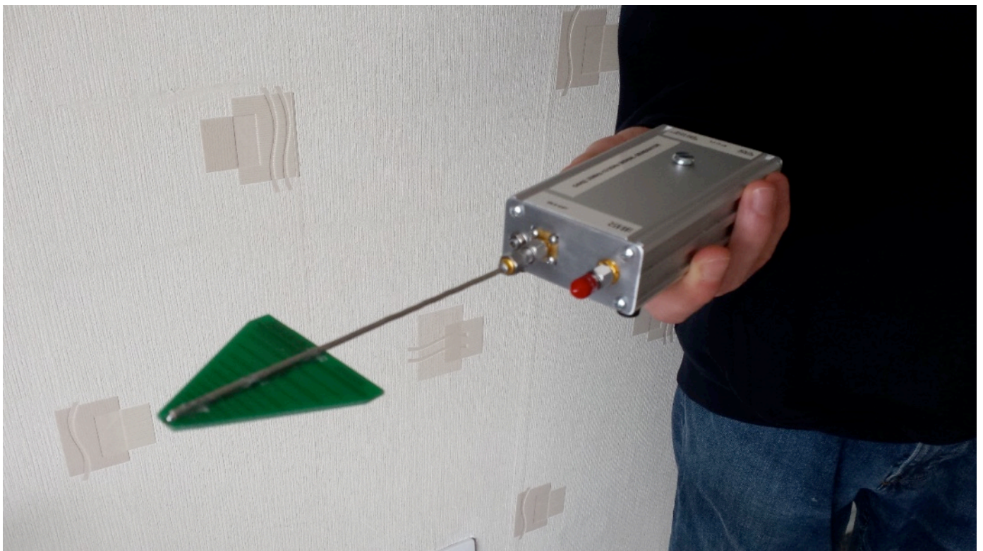
In use in hand-held mode, using a WA5VJB 2-11GHz antenna for 10GHz output.
