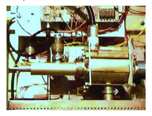
PCS Power Amplifier – before modification, PA Transistor above left end of blue power module
