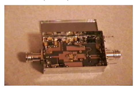
K9EK Amplifier in G3XDY 2.3GHz Transverter
