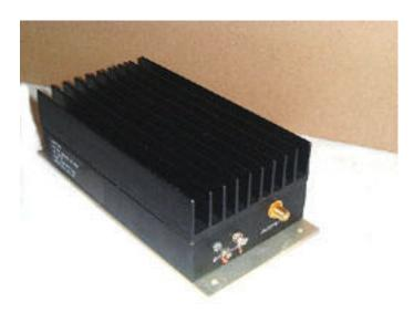
700MHz to 4.2GHz 1Watt output, 30dB gain, 1dB ripple broadband amplifiers.
