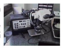
The trickiest bits are getting the force right and applying the energy. The first is solved with some simple mechanics and in modern machines, strain gauges. And with the second there are two main methods of bonding – thermosonic/ball bonding and thermocompression bonding.
