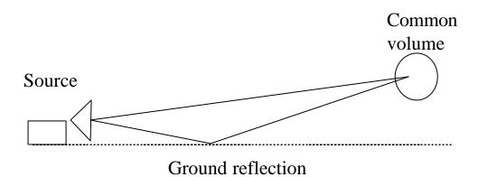
Figure 1 shows the ground reflection range with the source antenna close to the ground and the common volume in which the measurements are taken.
