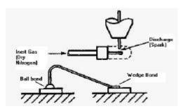
Ball bonding relies upon creating a blob of molten metal just a fraction of a second before the wire makes contact with the preheated die/track/package frame and then it is pressed down. Why pre-heated? If you think about it, putting a hot blob against a cold piece of metal isn't going to give an alloyed joint. This method of bonding is ideal for some devices and probably a large proportion
