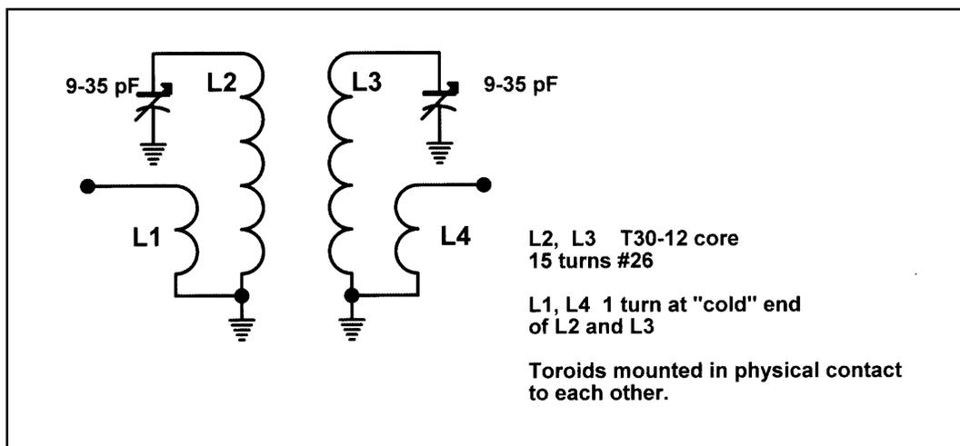
Figure 1. Double-tuned circuit.
