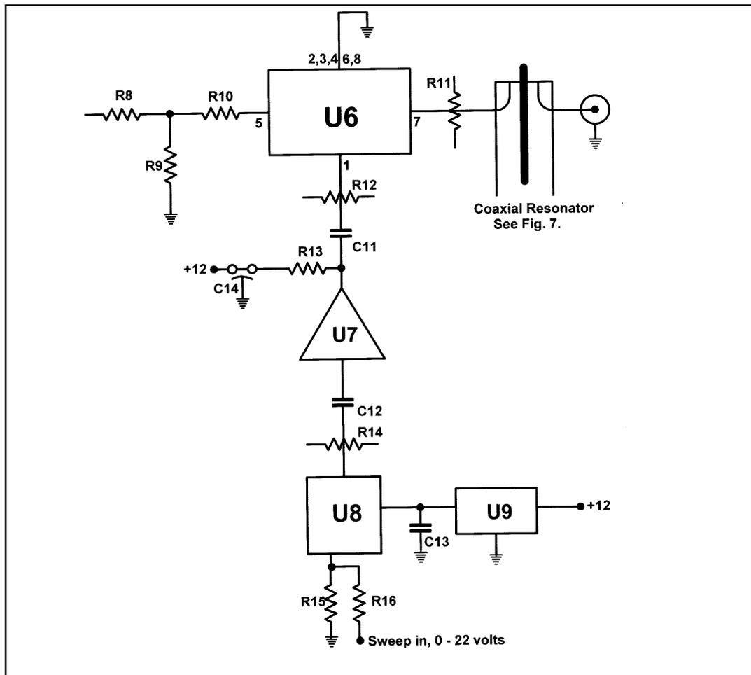
Figure 6. Converter using Wireless Radio model SM3-3000 VCO.
