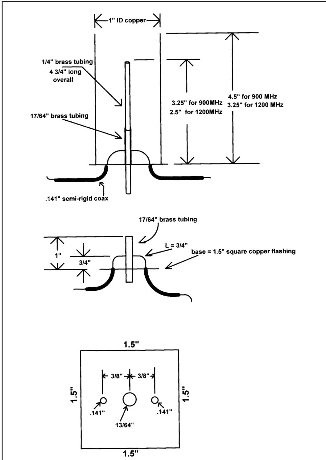
Figure 7. Coaxial filters.
