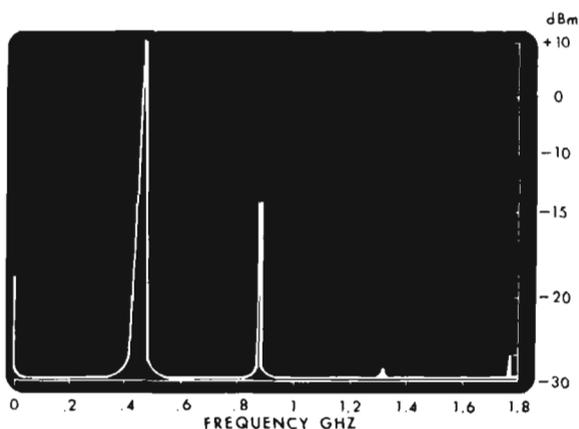
tudes are "stretched" somewhat, as seen in the scope photograph. However, it is possible to measure signal amplitudes to within one or two dB over the entire 40 dB range, once you get the hang of it. It is possible to view spectral components as far down as -40 dBm, but scale compression at the low end is so great that you can only guess at the actual amplitude.
