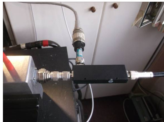
Fig.10. The power measurement setup using a 30dB directional coupler and 20dB attenuator giving 1kW F.S.D on the 10mW range of an HP432A power meter.
