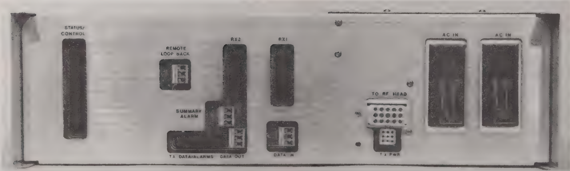
Figure 3-30. Hot Standby Switchover Unit – Rear View
