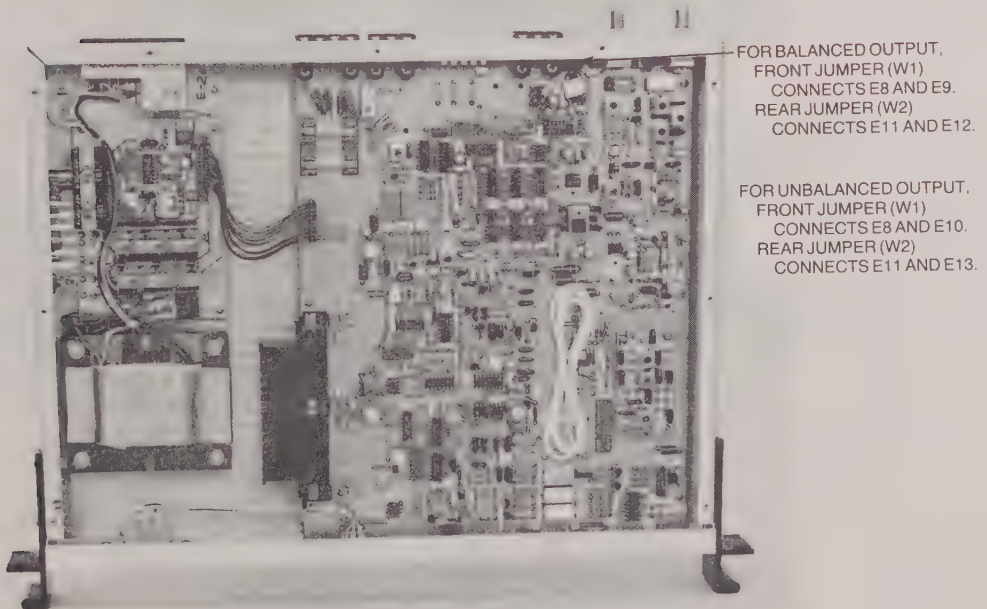
Figure 5-7. Receiver Board – Moving Jumpers To Change From Balanced Output to Coax, Unbalanced Output
