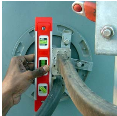
Figure 5-1. Checking Feedhead Flange with a Spirit Level
