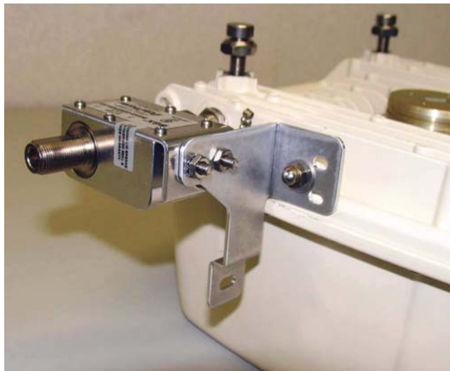
Figure 2-27. Universal Support Bracket: Horizontal Suppressor Installation
