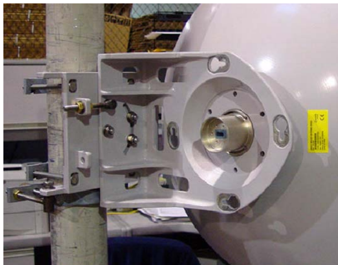
Figure 2-7. Precision Pole Mount and ODU Mounting Collar
