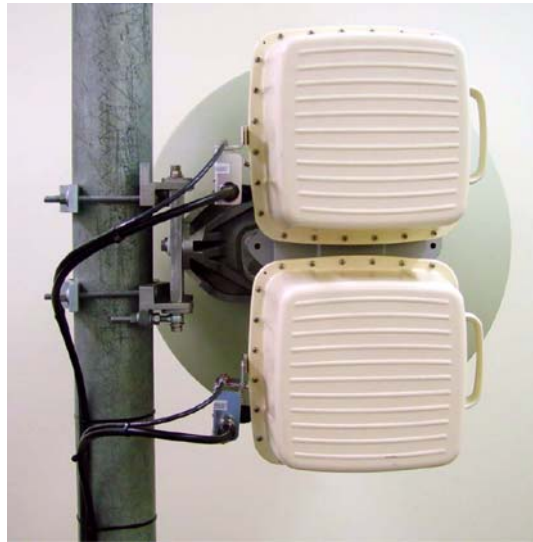
Figure 2-19. Vertical Coupler Installation with ODUs: Rear View
