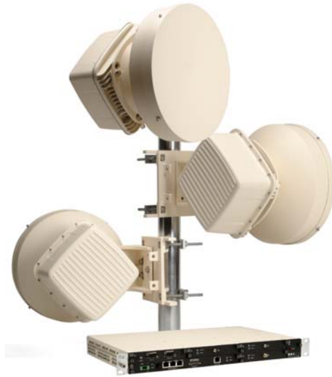
Figure 1-8. Eclipse Node: INU with Three ODUs
