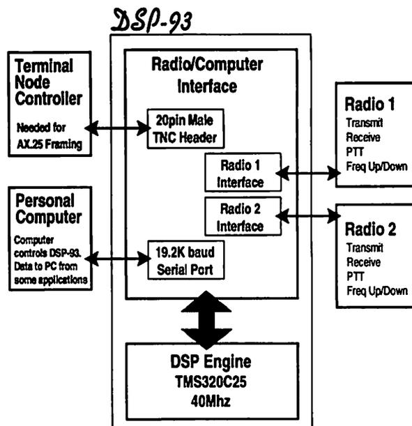
Interface Board, top board, contains two eight-pin female mini-DIN connectors for radio interfacing. Incoming radio signals pass through a voltage divider to establish the initial levels, then through an eight-channel multiplex chip. The multiplex chip then feeds the single A/D input with either of the two radio inputs or one of the six auxiliary inputs. The Texas Instruments TLC32044
