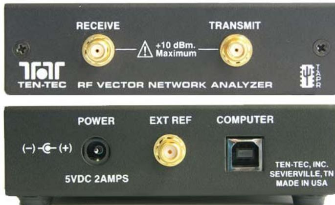
Designed for testing up to 100 MHz, the unit connects to your PC via USB and the software runs on Windows-based systems.
