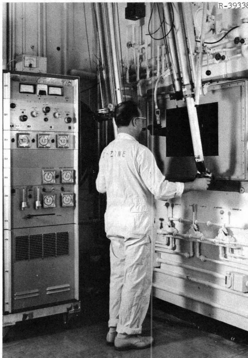
Fig. 1. Setup at cell window for gas tungsten-arc welding.
