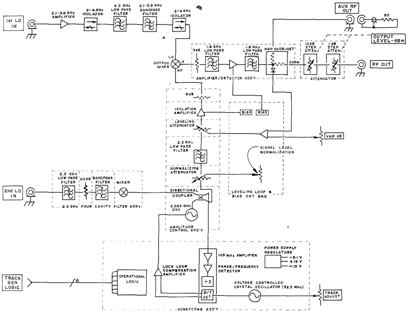
Fig. 1. Block diagram of the TR 502 Tracking Generator.
