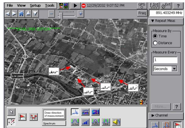
Figure 15. GPS mapping capability significantly helps narrow DF information to home in on transmitter locations.
