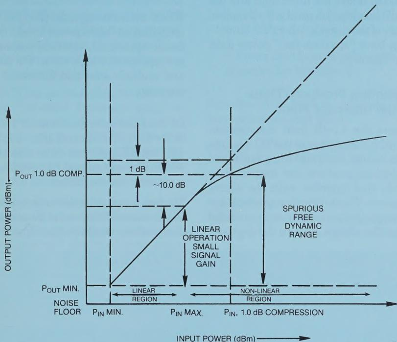
**Figure 8. Linear/non-linear power response.**
