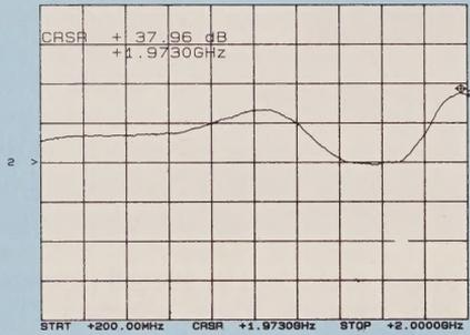
Figure 6C. A31/1/RA36 cascaded gain response.
