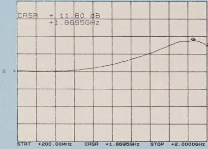
Figure 6A. WJ A31-1 amplifier gain response.
