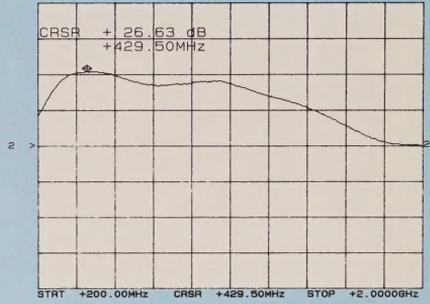
Figure 6B. WJ RA36 amplifier gain response.
