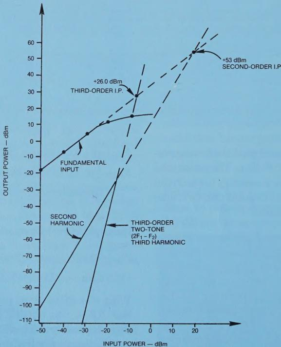
Figure 10. Output power vs. input power for the A31-1/A35/A37 cascaded amplifier.
