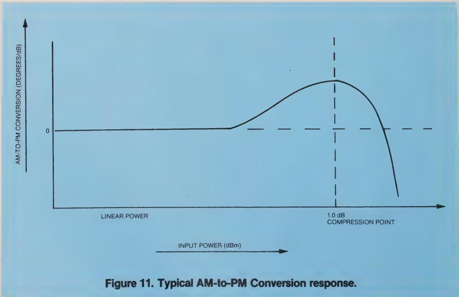
**Figure 11. Typical AM-to-PM Conversion response.**
