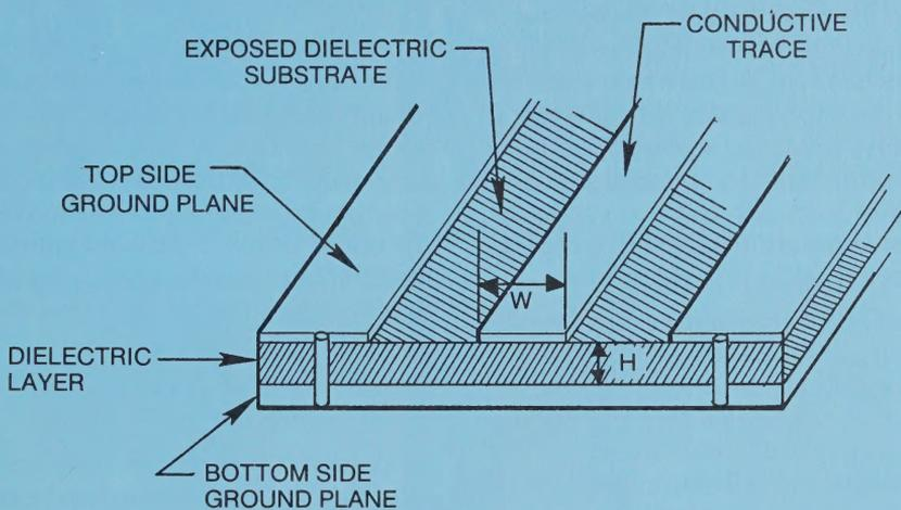
Figure 2. Printed-wiring board description.
