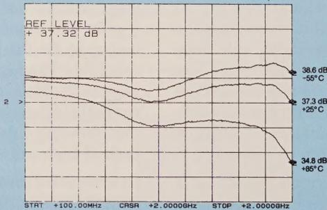
Figure 7. Cascaded amplifier performance over temperature.
