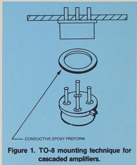
**Figure 1. TO-8 mounting technique for cascaded amplifiers.**
