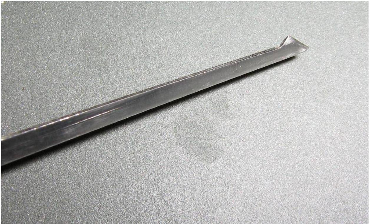
Picture showing some of the high spots being removed from the lock pick. Note the sanded areas near the tip of the lock pick.
