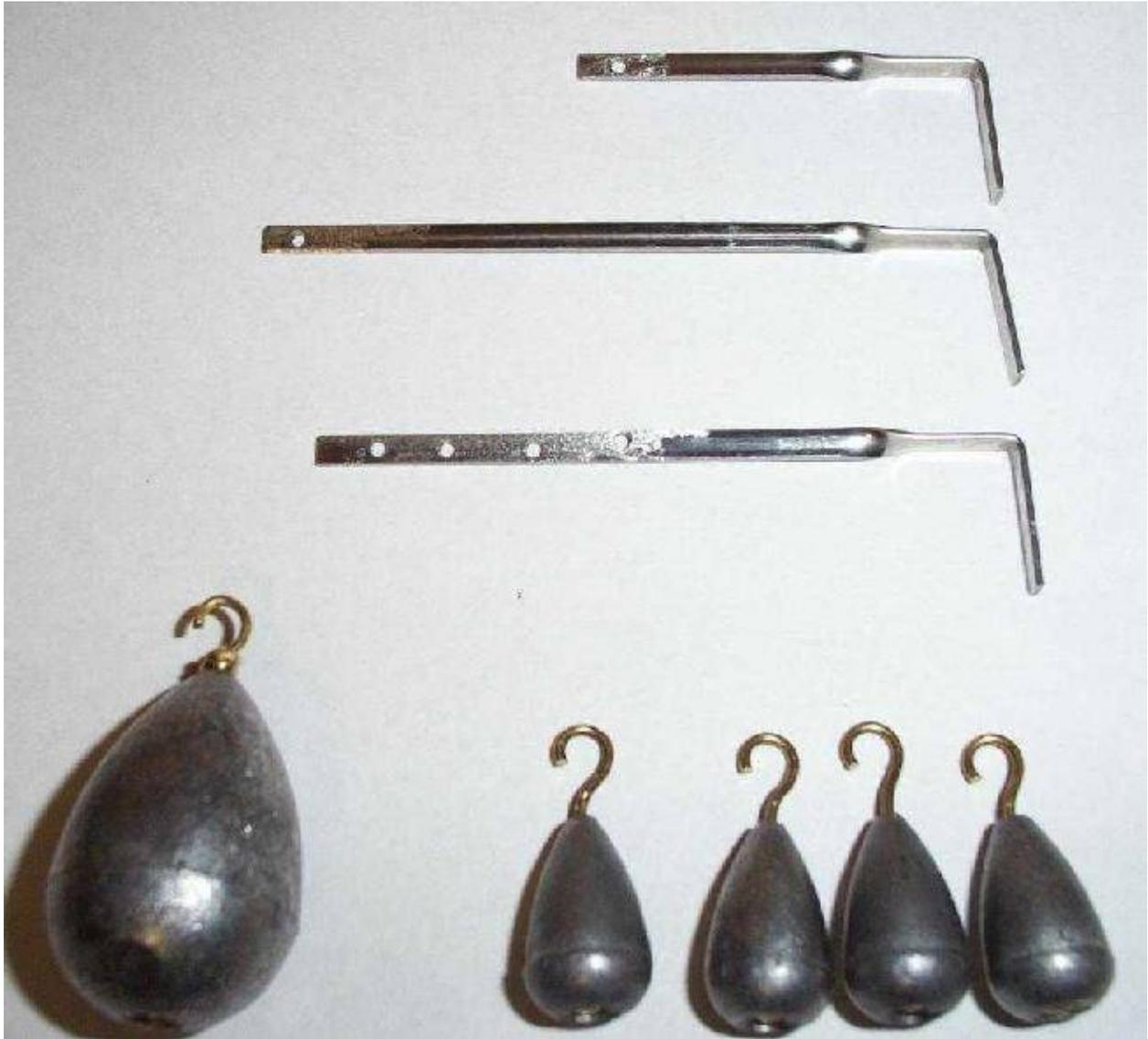
You can also do the same thing by drilling holes into the tension wrench and adding slightly modified lead fishing sinkers. Trim the eye hooks so they are removable. Experiment with different size sinkers and tension wrench hole positions.
