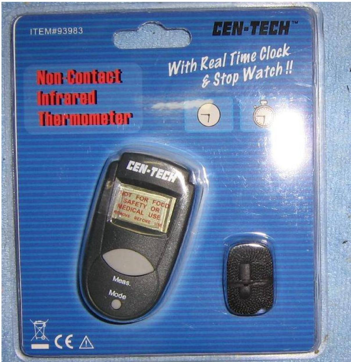
You can experiment a bit with a *much cheaper* alternative. The idea is to use a Cen-Tech Non-Contact Infrared Thermometer (Harbor Freight Tools #93983) to measure the ambient keypad's temperature, then quickly remeasure the key's temperature after it has been pressed. This overall idea still needs a little tweaking, but it does appear to work.
