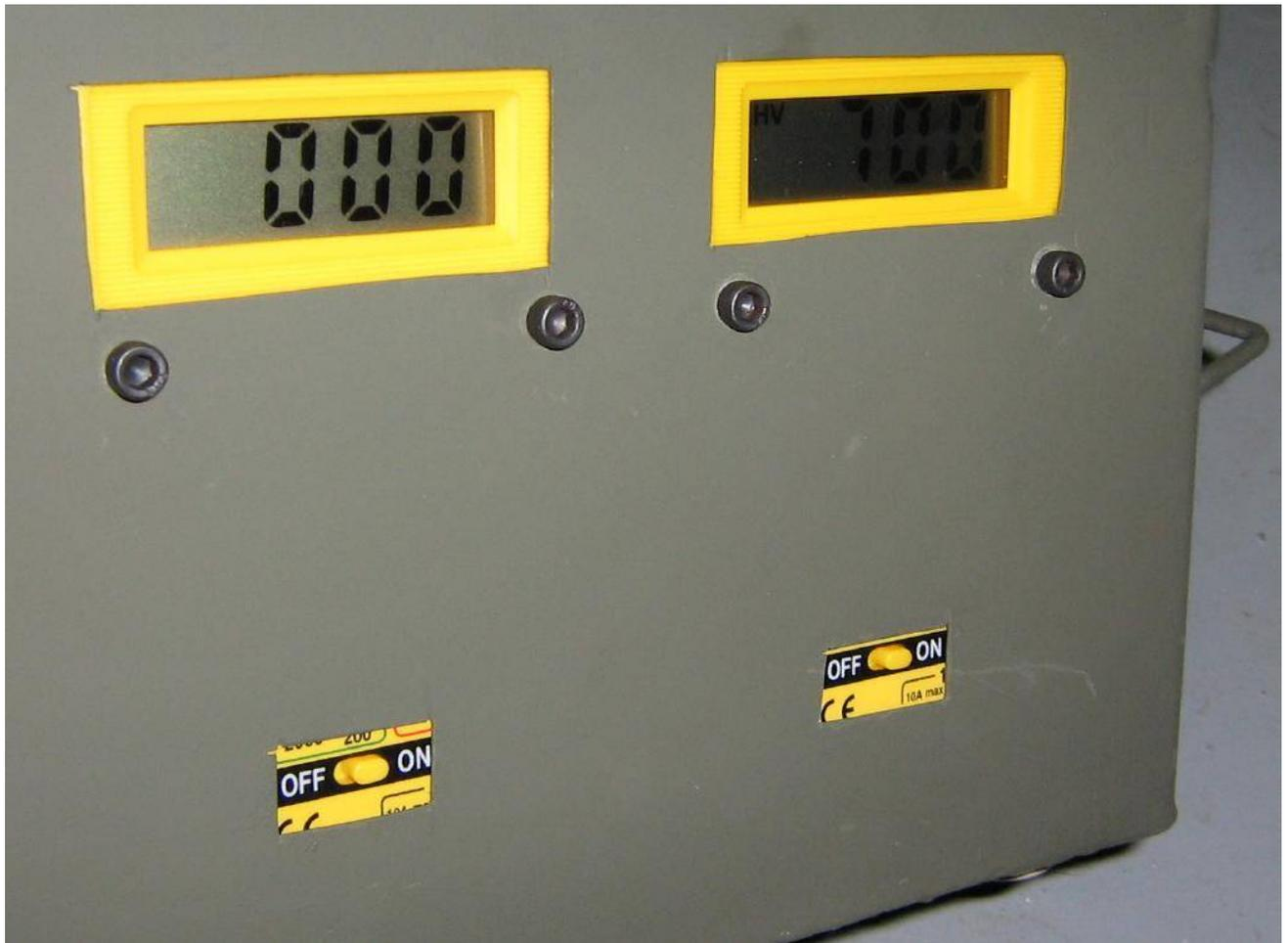
Main power is on. Meter close up picture. The meter on the left is reading the current draw (none) and the meter on the right is reading the high-voltage output (700 volts).
