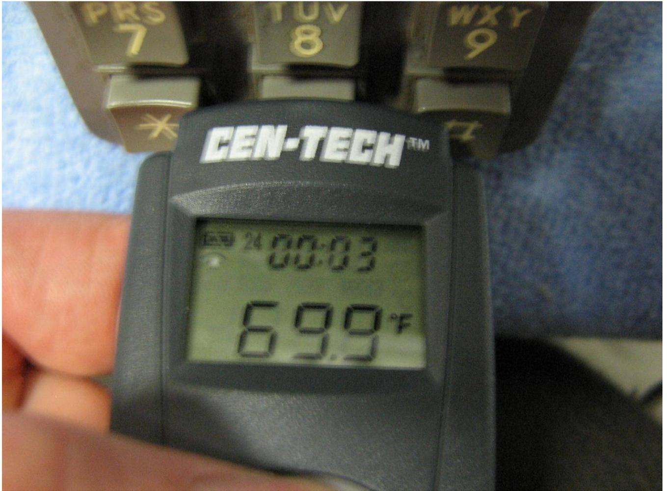
Testing. The Non-Contact Infrared Thermometer is held against a key to measure its ambient temperature, 69.9°F in this case.
