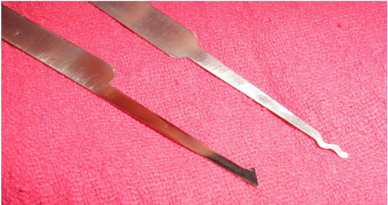
After the pick has been sanded, you can then perform the final step of polishing the pick to a mirror-like finish. Apply some polishing compound to the buffing wheel in the Dremel tool and lightly work both sides of the lock pick.
