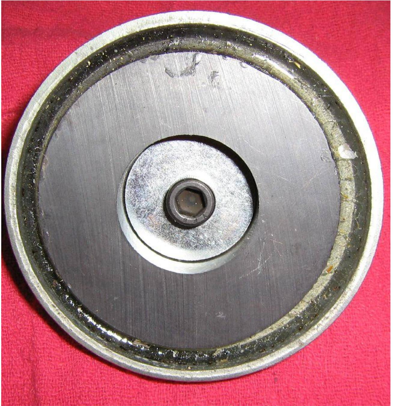
Bottom view. Put it together like this with one fender washer on top and one on the bottom with the coupling nut and bolt holding everything together. Secure everything very tightly.
