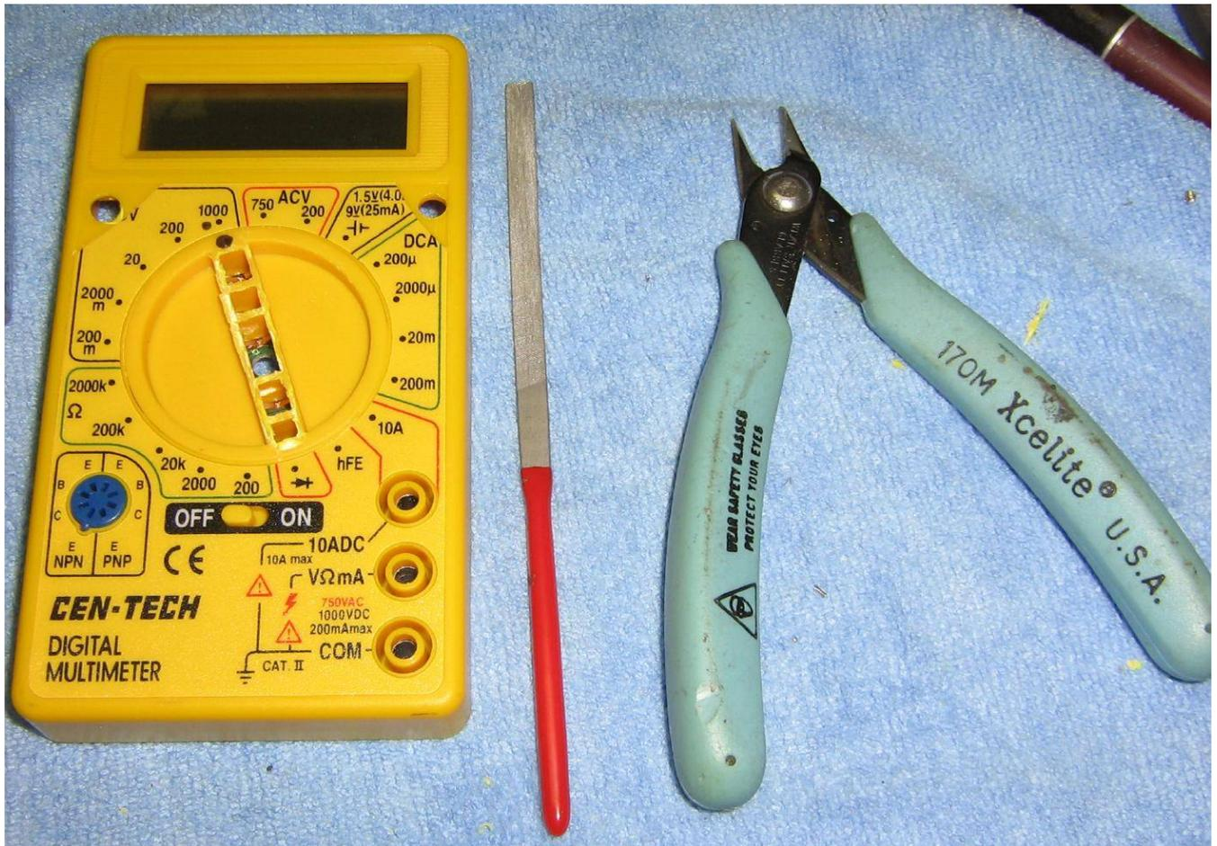
Cut and file down the large plastic selector switch on the meter's front so it can rest along the inside of the project case. Leave the on/off switch as it is.
