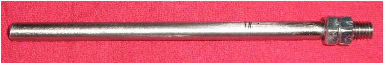
It should look something like this when finished. Use two "jam" nuts on the threaded end to secure the rod into the coupling nut. You will also want to polish the steel rod with some fine sandpaper or steel wool.
