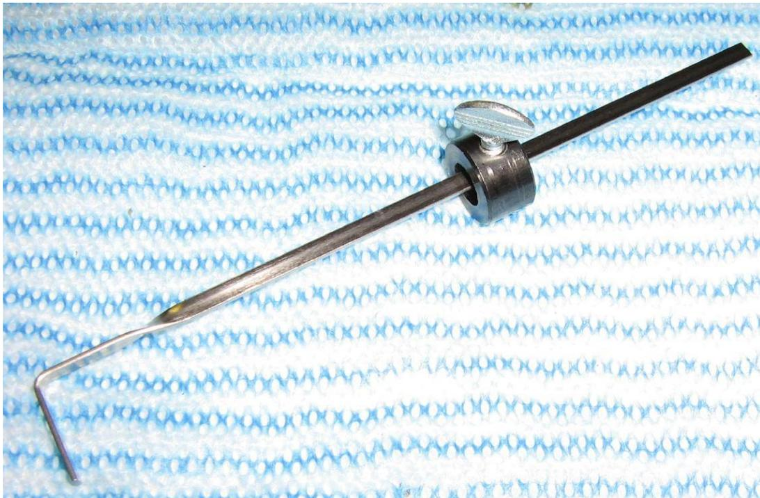
In operation. Slide the weight up or down the wrench for the proper turning pressure. Add more weights if you need more pressure.
