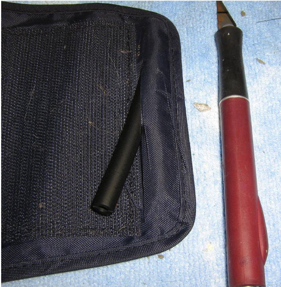
The only real modification, besides removing the electronics and shortening the inflator tube, is to remove the little rubber end piece on the arm cuff. This will allow it to slide more easily underneath doors with a narrow gap.
