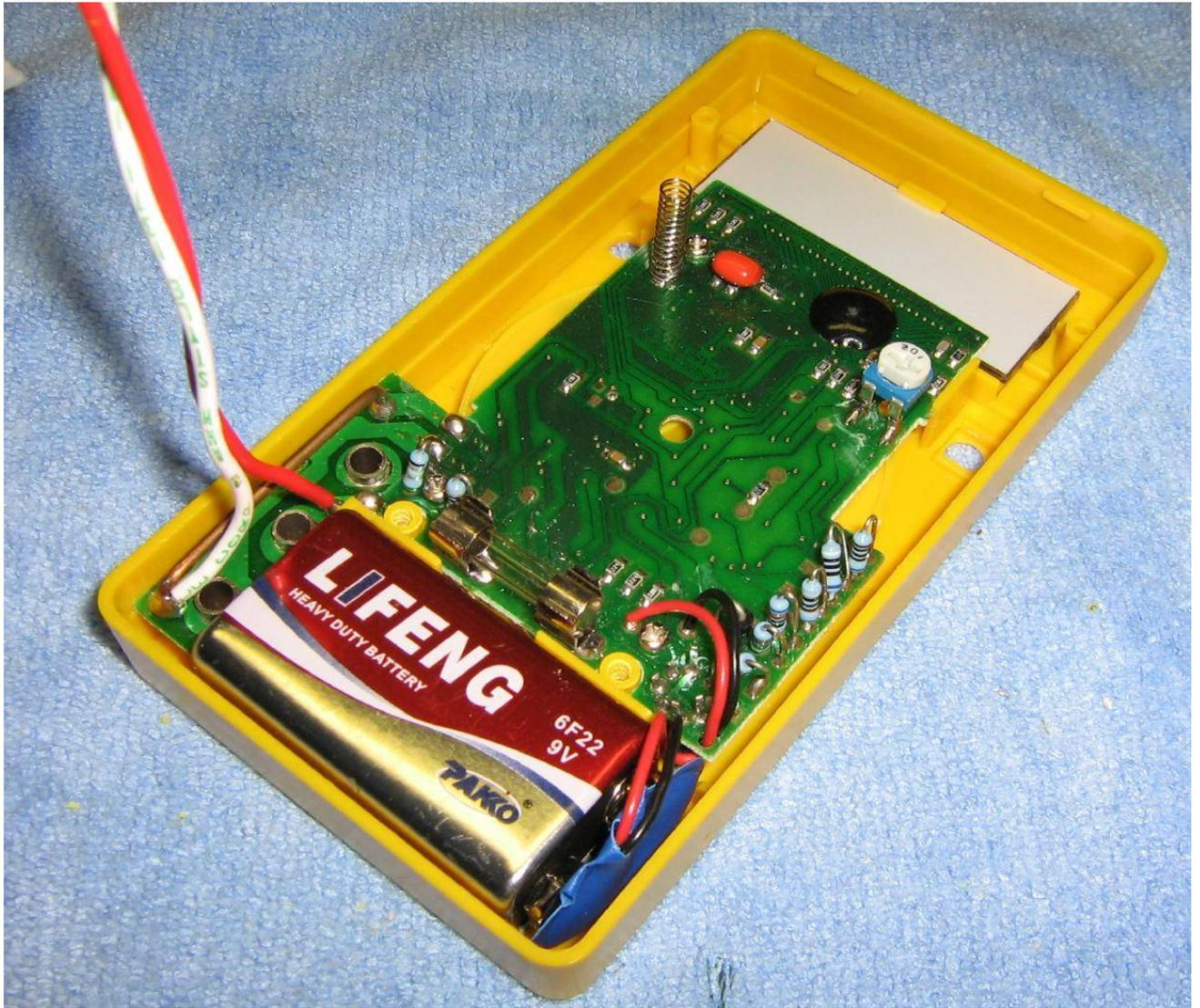
Inside of the meter. Solder two wires to the meter's terminals. Both the meters can be soldered in the same place. Drill a hole on the rear cover to pass the wires through.
