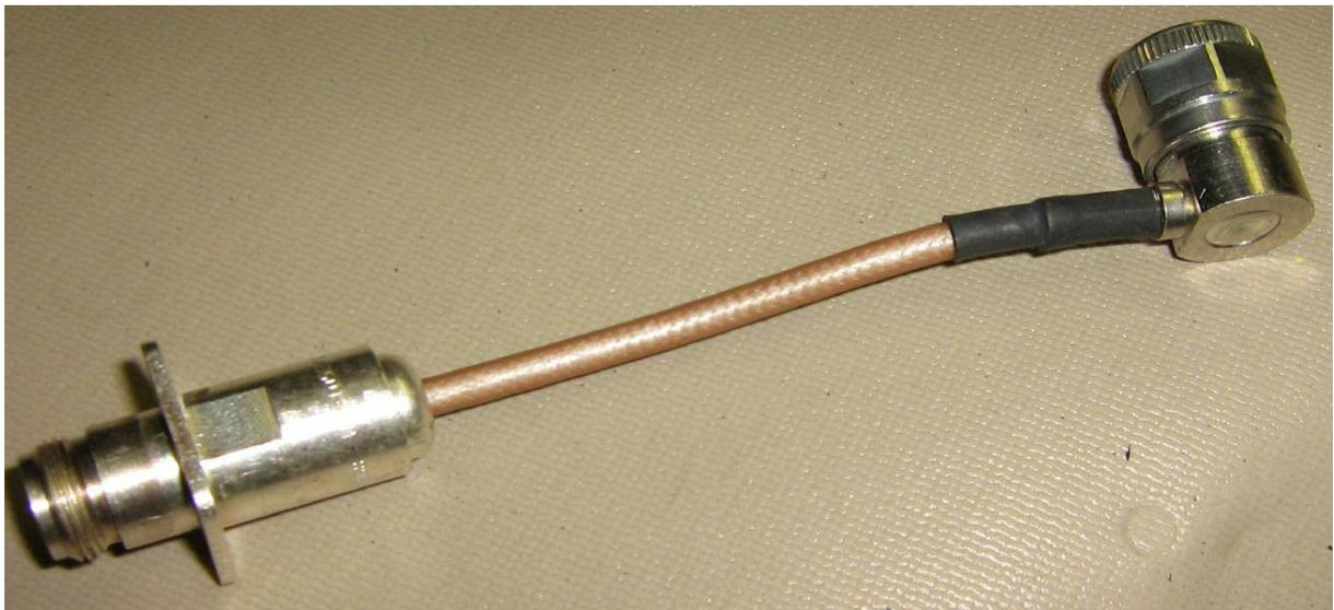
RF output coaxial assembly. Front-panel female N connector connects to a right-angle male N connector with a piece of Teflon dielectric RG-142 coax.
