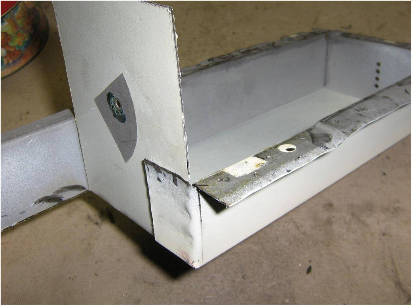
Sheet metal waveguide section salvaged from an old 1980s microwave oven. For this project, you'll need one at least 8 inches long.
