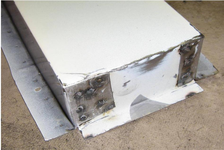
Cut and fold over the open end of the waveguide so it is exactly 7.5 inches (19 cm) long. This is equal to *one waveguide wavelength* at 2.45 GHz. Try to get ahold of a spot welder to secure the sheet metal flaps. Use rivets or epoxy as a last resort. Harbor Freight Tools has a spot welder (#45689) which works nicely on standard 120 VAC wiring.
