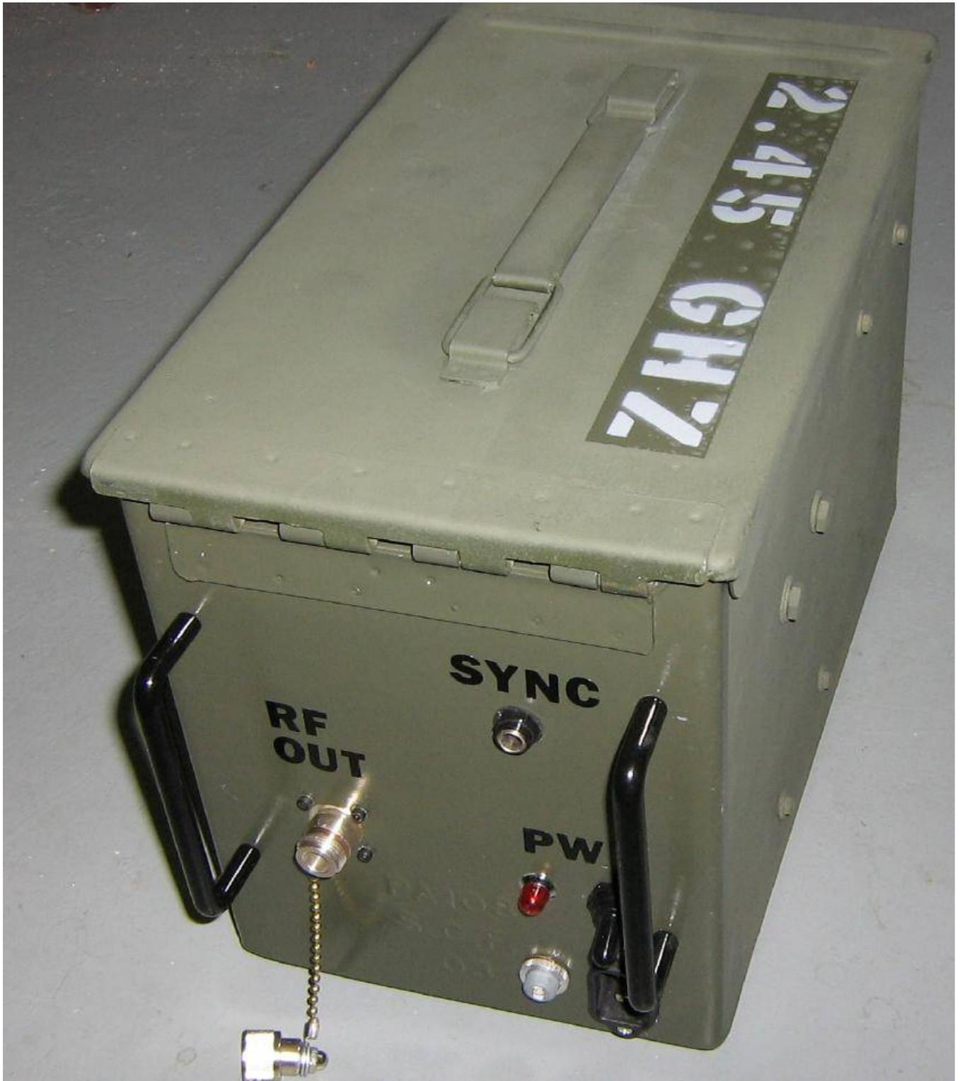
Outside front-panel overview. The **SYNC** output is a 1/4 inch stereo jack and is isolated from the front-panel using a rubber grommet.
