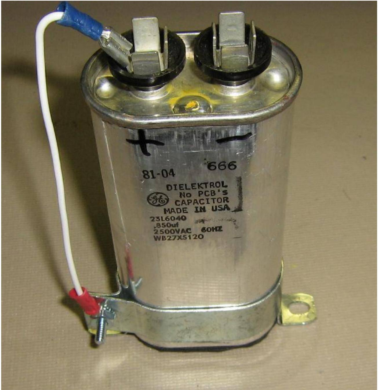
High-voltage capacitor from an old microwave oven. The "positive" side is connected to ground.
