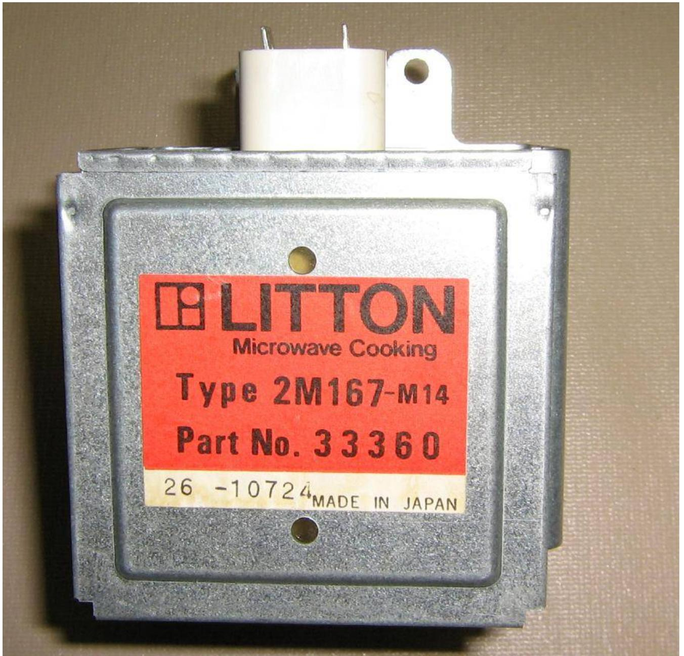
Magnetron used for this project. It's a Litton 2M167-M14. It appears to do around 800 watts CW at 2.45 GHz.
