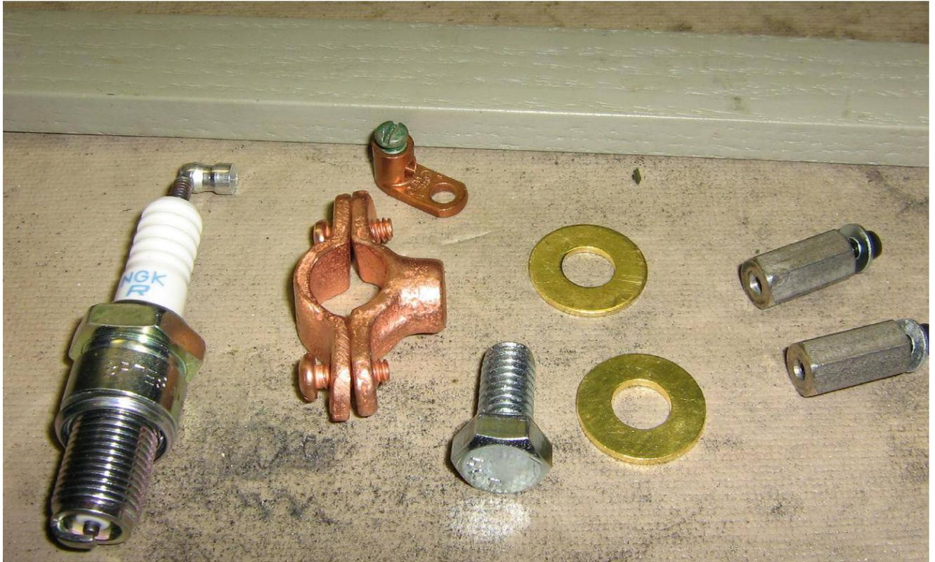
For this project, which is intended to be used as an experimental radar system, we'll be pulsing the magnetron using a spark plug. The spark plug will be secured to a wood insulator using a 1/2 inch copper split-ring hanging clamp. The main thread in the camp is standard 3/8-16. A small ground lug will connect the pulse wiring to the clamp's body.
