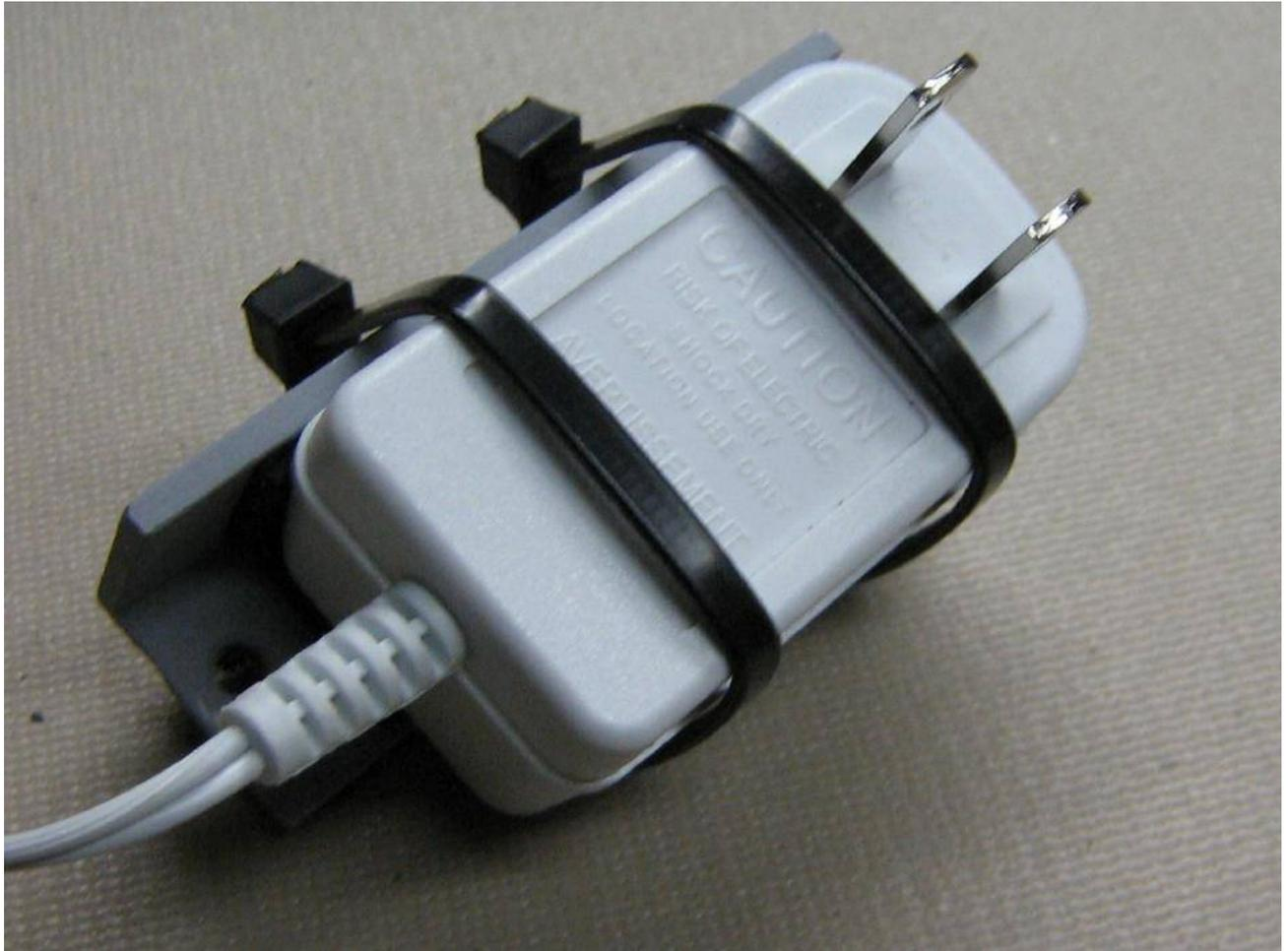
Find an old 12 VDC wall-wart power supply and secure it to a L-bracket. This will be used to power a small fan mounted above the magnetron. Solder the incoming 120 VAC wires directly to the wall-wart's prongs.
