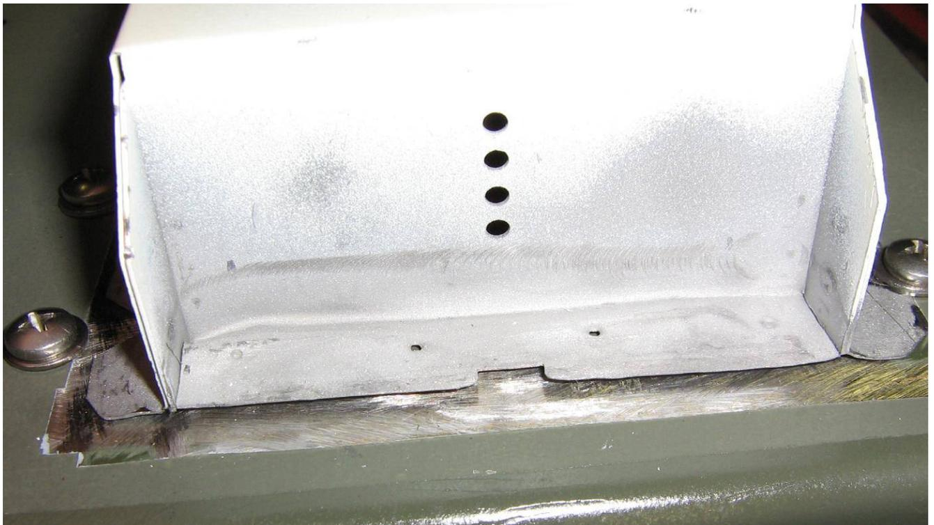
A minor problem securing the waveguide will be around the section where the magnetron is located. It's not possible to use rivots without drilling clearance holes in the magnetron's body. You may wish to use some two-part epoxy putty to secure the sheet metal flaps down.
