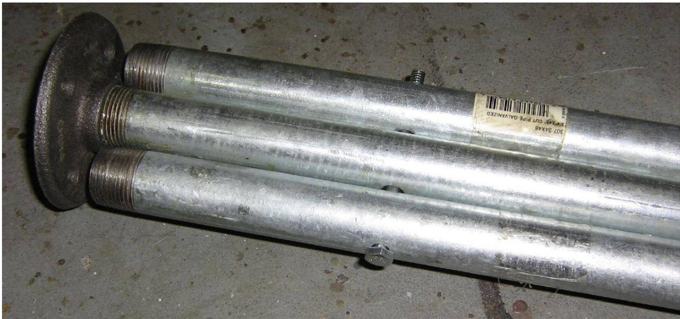
To store the mast sections during transport, drill holes through each of the 3/4-inch pipes near each end. Place a large 1/4-inch threaded bolt through them and secure with wing nuts.
