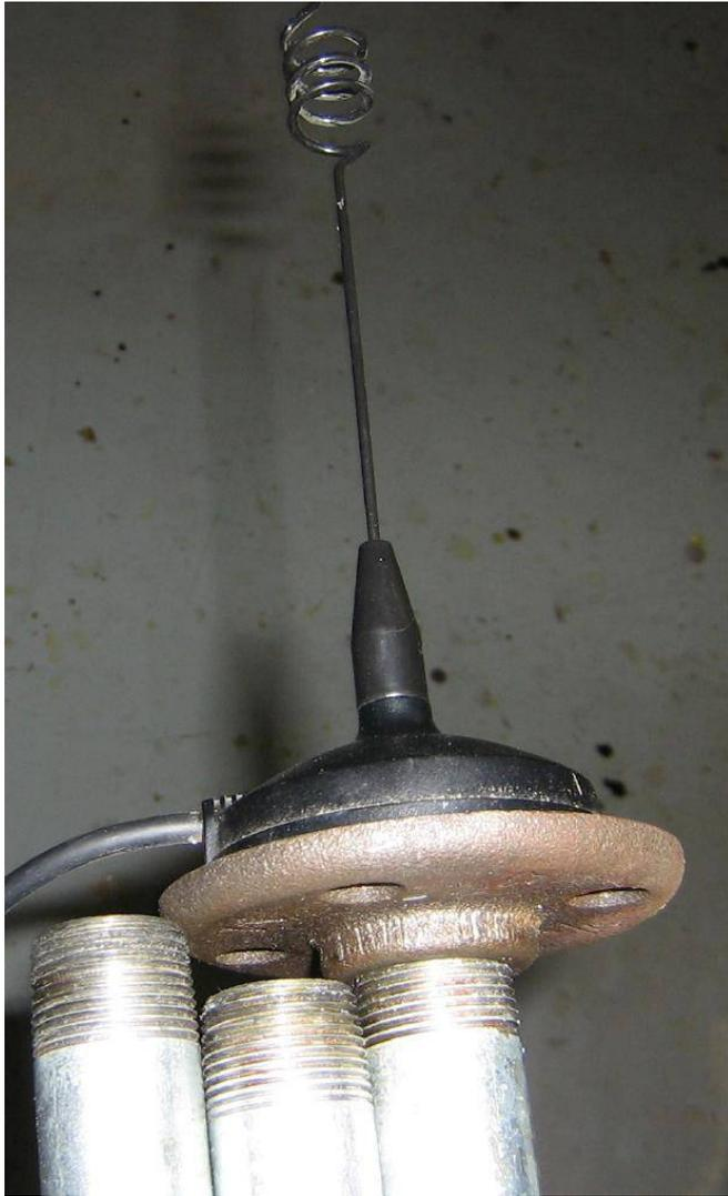
Another 3/4-inch floor stand can be attached to the top mast piece to make a platform for a magnetic mount antenna.
