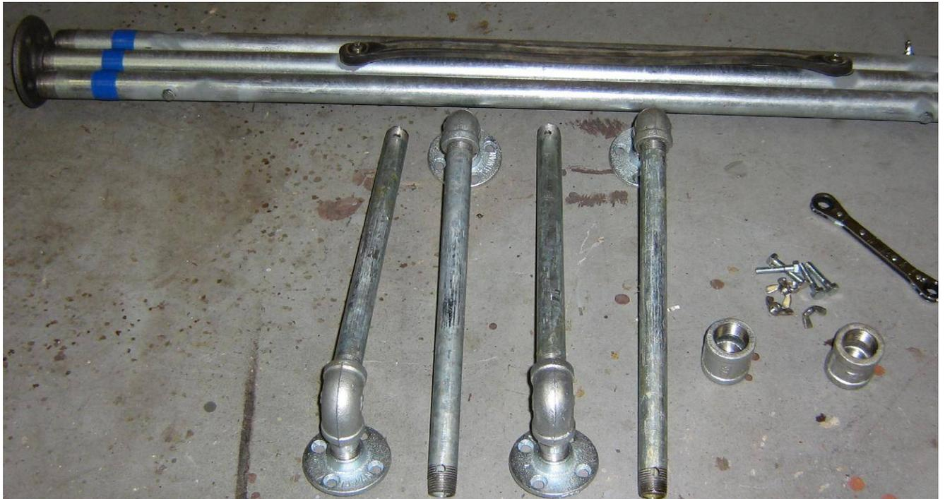
Completed portable antenna mast system.
