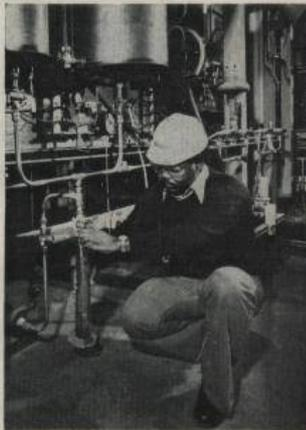
TECHNICIAN at Mobil lab taps gasoline from methanol, which can be coal-derived.
