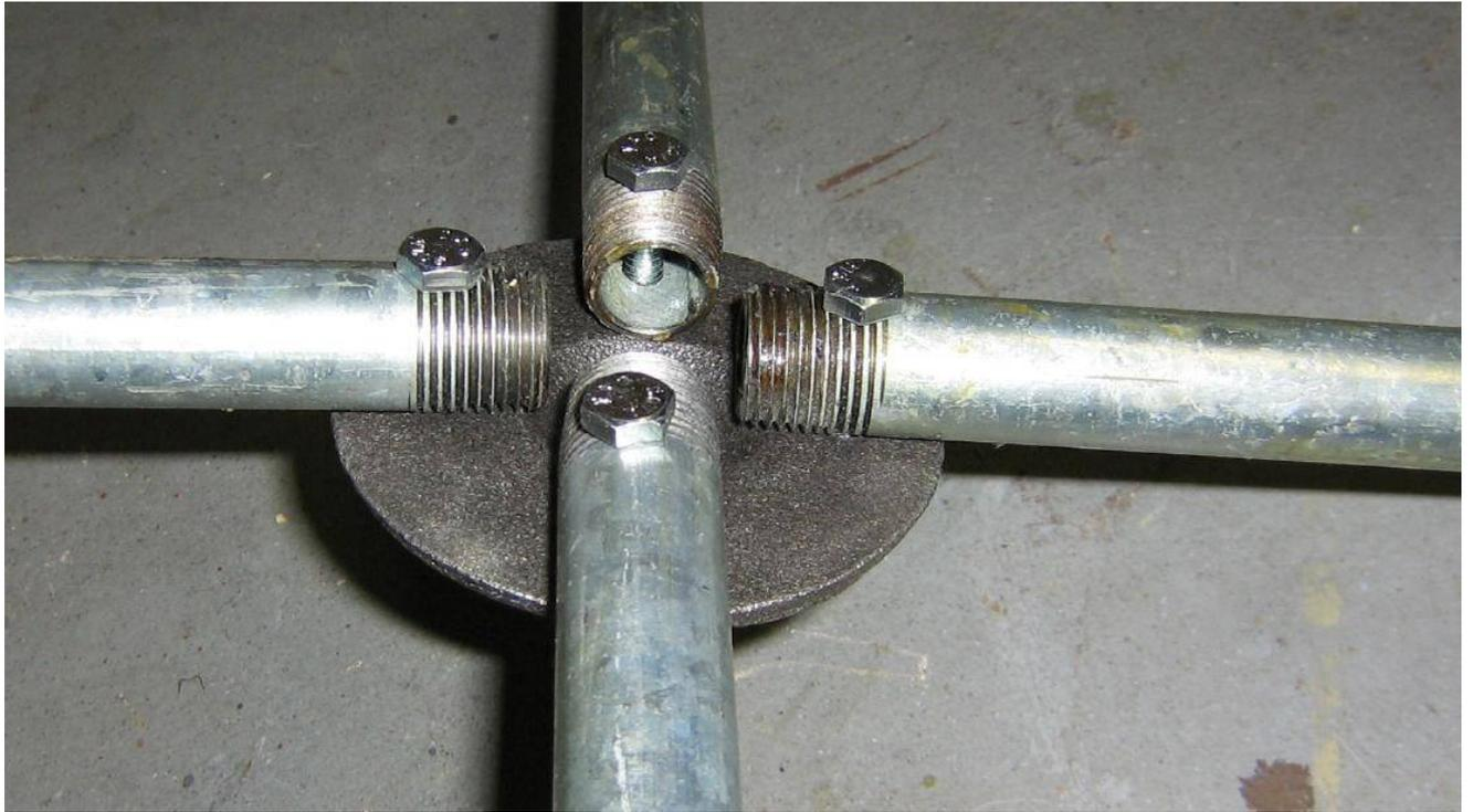
After you've made the four legs for the mast stand, drill a 1/4-inch hole through one end of the 1/2-inch diameter pipe, as shown above. This is how the legs will attach to the 3/4-inch floor stand which supports the main mast itself. Secure the legs using the 1/4-inch hardware.
