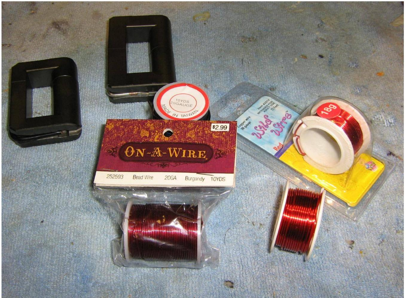
The enameled wire we'll be using and some example ferrite cores on the upper-left.
