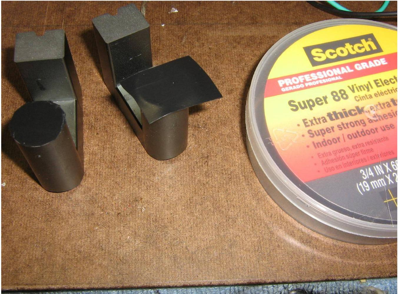
In order to keep the ferrite core from saturating, you can add a small air gap to one of the core's legs.
