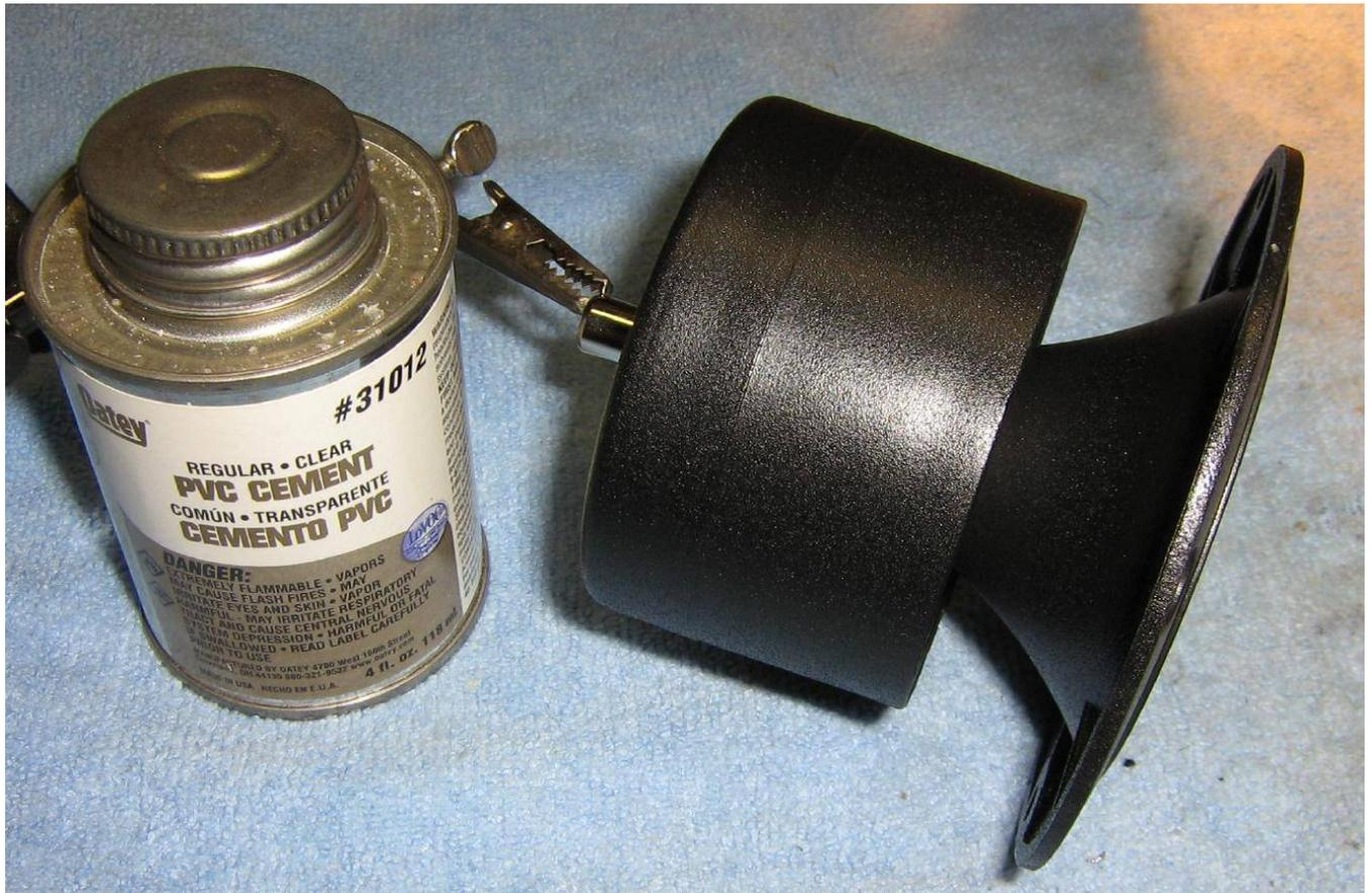
Slide the piezo horn tweeter into the 2-inch cap and secure using PVC cement.
