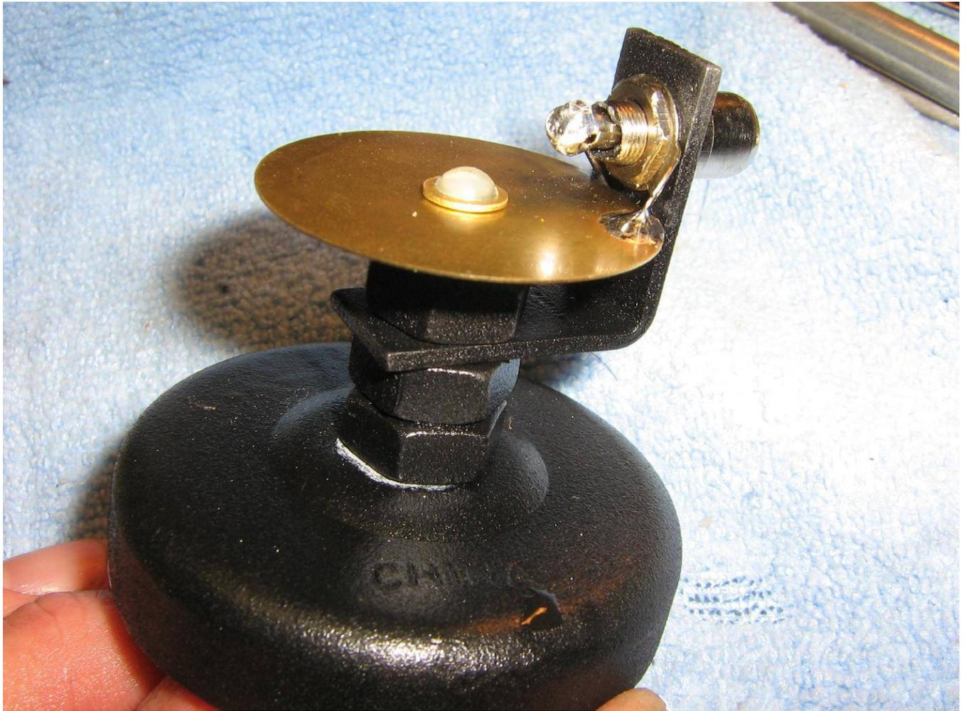
Completed magnetic-mount contact microphone.
