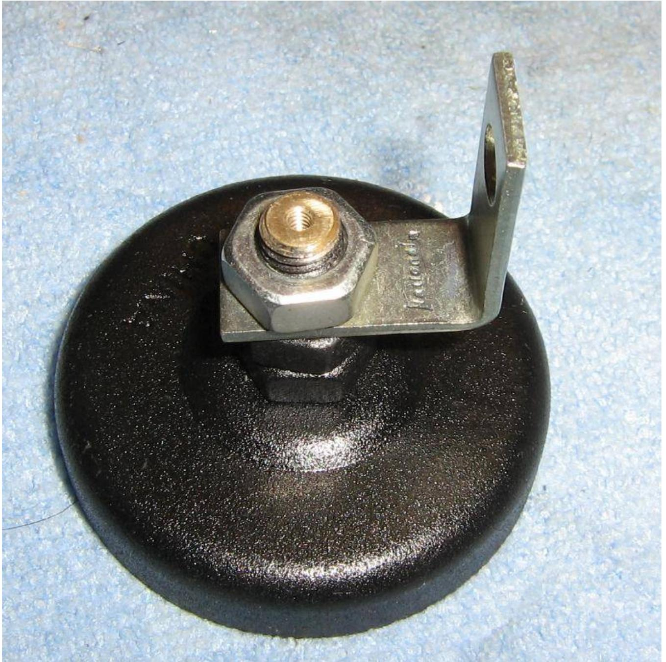
Mount a small L-bracket to the threaded brass stud of the magnetic ground block, as shown above.
