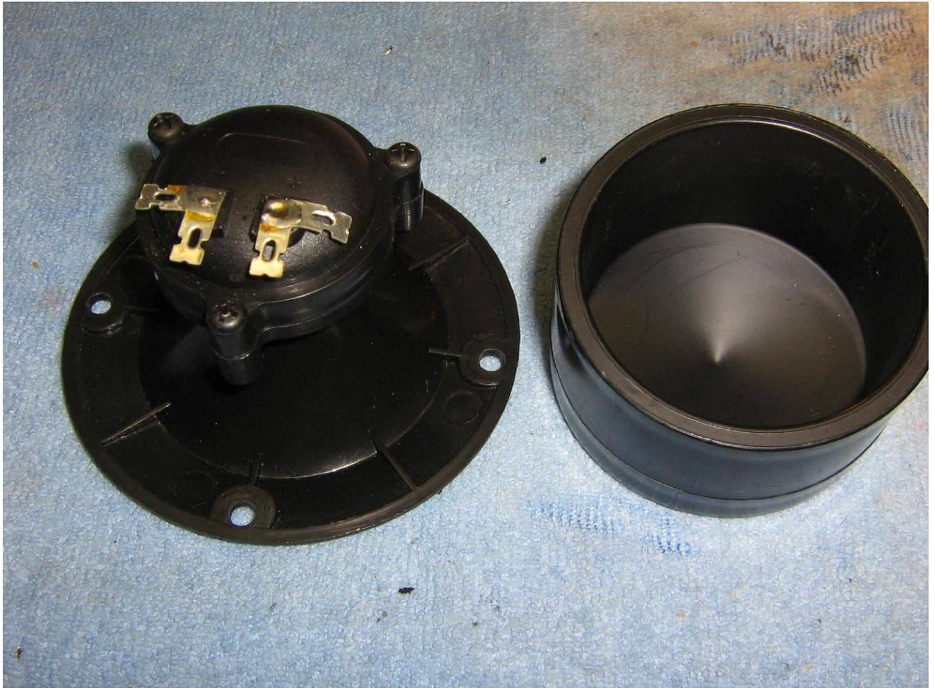
Rear view of the piezo horn tweeter showing the contacts.
