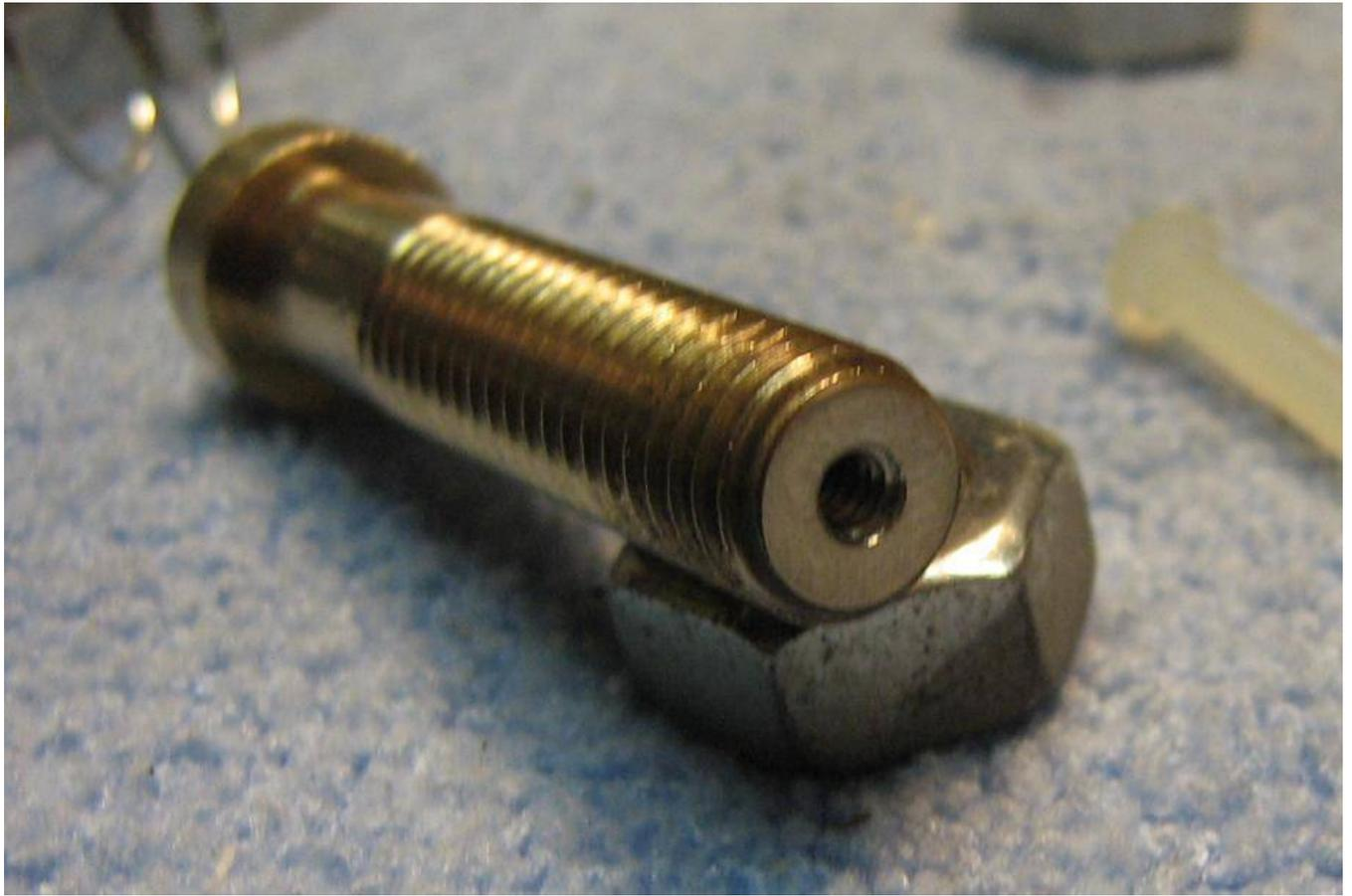
Very carefully drill and tap a #4–40 screw hole in the center of the "threaded end" of the magnetic ground block's brass stud.
