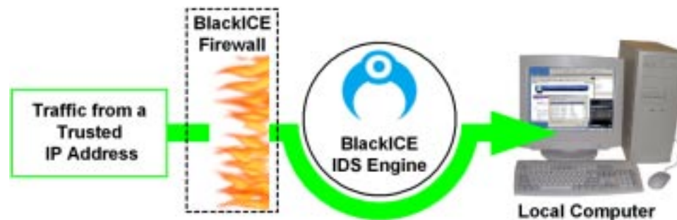
Figure 4 – Trusted traffic is still eligible for firewalling, but is not analyzed for intrusions.
