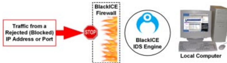
Figure 6 – Rejected (Blocked) traffic is stopped at the BlackICE firewall.
