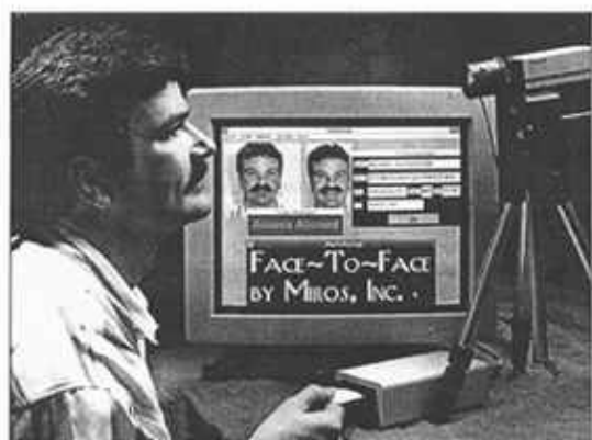
Face-To-Face uses a video camera to match a person's face with a stored image on an electronic ID card.
